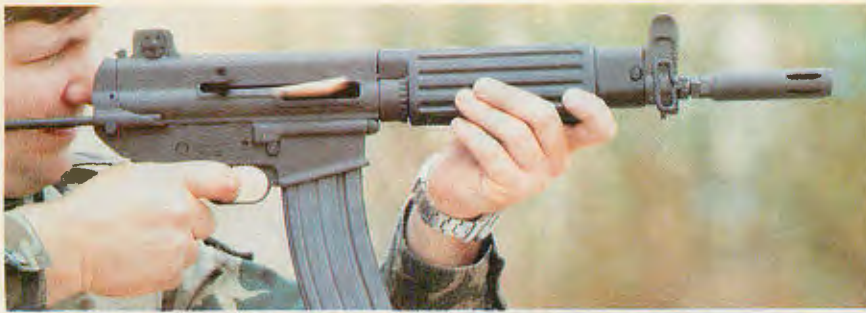
LEFT: For no known reason, Daewoo has chosen a different, Ljungman-type gas system for its carbine.
